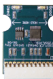
P/N - CM255B Panel Default Unlock Key Will reset Installer PIN and RAS PIN on Solution 6000 panels.
