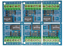
P/N - CM940B 6 Way Programmable Relay Card. Can be separated into single relay cards.
